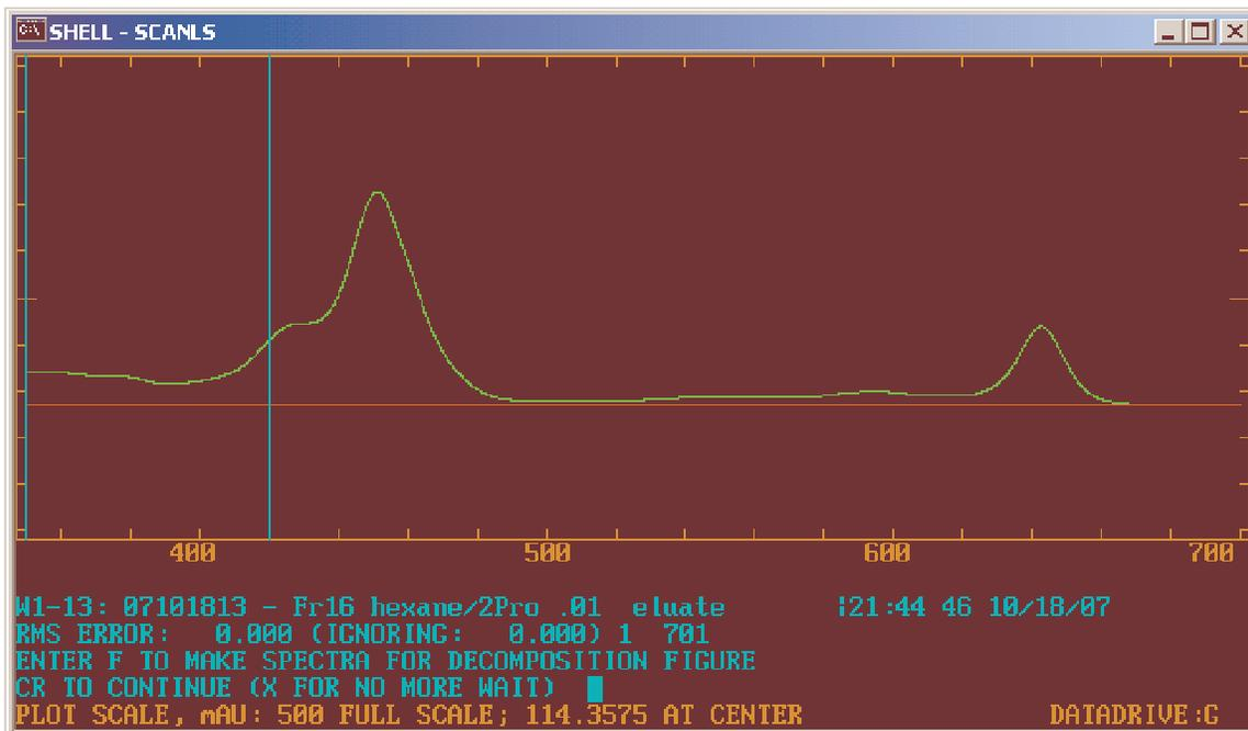
Spectra 14 and 15 do not fit adequately. Clearly another component is present. Also 15 is in acetone not hexane, which affects the spectra.
