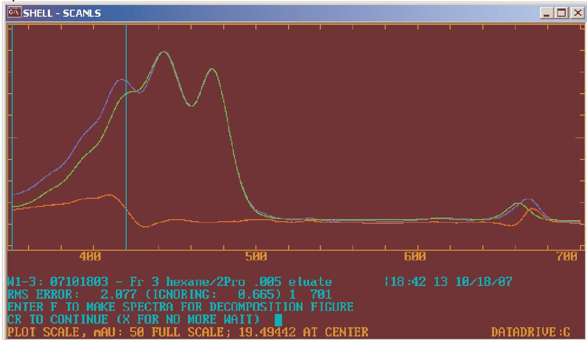
Spectra 4 to 13 fit well, apparently no other component is eluting here. Carotenoid peaks in
